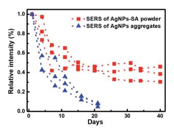
Fig. 4 SERS stability of the AgNPs-SA powder. Squares and triangles demonstrate the SERS intensity ( $l_{1436~cm^{-1}}$  of 4-ATP) evolutions of 3D AgNPs-SA powder and conventional 2D AgNPs aggregates with different preserved time in ambient condition, respectively. For comparison, three groups of controlled experiments were done. The dash lines are plotted to guide eyes.
