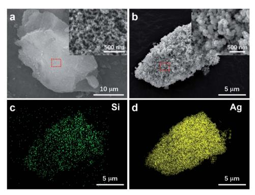
Fig. 1 The surface morphology and elemental analysis of the AgNPs-SA powder. (a) The SEM image of the silica aerogel particle. The inset shows the corresponding magnified image. (b) The surface morphology of the synthesized AgNPs-SA. The inset shows the corresponding magnified image. (c) and (d) The elemental mappings of AgNPs-SA composite in (b) by using Si and Ag, respectively.
