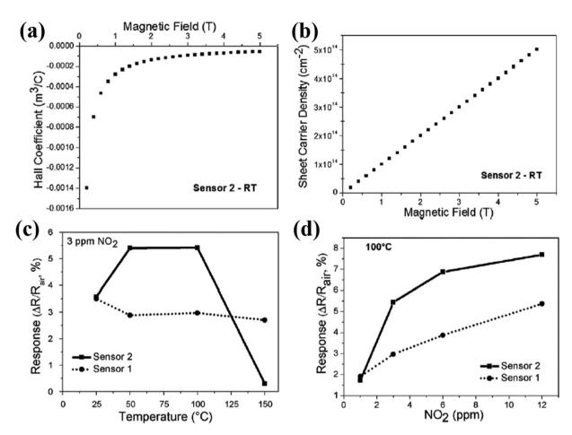
Fig. 6 (a) Hall coefficient. (b) Sheet carrier density of the as-deposited galinstan film (Sensor 2,  $10 \mu m$  thickness). (c) Response of the as-deposited sensors towards 3 ppm  $NO_2$  as the function of the operating temperature. (d) Response amplitude of the as-deposited sensors as a function of  $NO_2$  concentration. Reprinted with permission from ref. 48. Copyright (2017) Elsevier.
