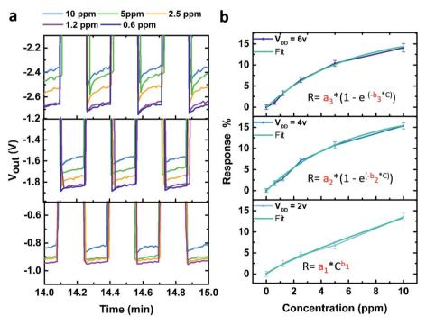
Fig. 3 (a) Output voltage of the inverter after exposure to various concentrations of NO<sub>2</sub> gas for a  $V_{\rm in}$  at -4 V and -11 V alternatively for three different  $V_{\rm DD}$  values (from top to bottom:  $V_{\rm DD}=6$  V, 4 V and 2 V). (b) Response of the inverter as a function of NO<sub>2</sub> concentration for the three different  $V_{\rm DD}$  values (from top to bottom:  $V_{\rm DD}=6$  V, 4 V and 2 V).
