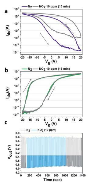
Fig. 2 (a)  $I_{ds}-V_{g}$  characteristic of the p-type SWCNT-FET before and after 15 min of  $NO_2$  exposure ( $V_{DS} = 1 \text{ V}$ ). (b)  $I_{ds} - V_g$  characteristic of the n-type SWCNT-FET before and after 15 min of  $NO_2$  exposure ( $V_{DS}$  = -1 V). (c) Output voltage as a function of time of the inverter under an exposure of  $NO_2$  gas for a square input voltage for alternatively -4 Vand  $-11 \text{ V} (V_{DD} = 2 \text{ V})$ .
