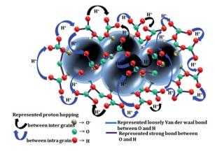
Fig. 4 Inter- and intra-grain proton-hopping model.
