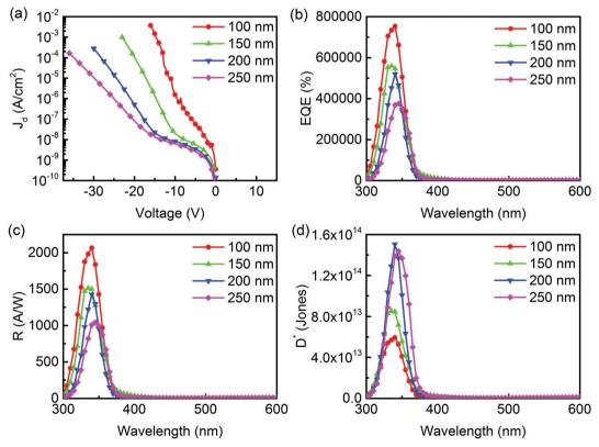
Fig. 4 (a)  $J_d$ , (b) EQE, (c) R, and (d)  $D^*$  characteristics of the fabricated UV PM-type OPDs with different active layer thicknesses. The device structure is ITO/TAPC:  $C_{60}(50:1, 100 \text{ nm}, 150 \text{ nm}, 200 \text{ nm}, 250 \text{ nm})$ /Al (100 nm).
