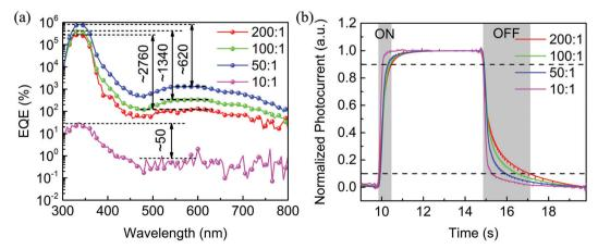
Fig. 6 (a) EQE and (b) transient photocurrent responses of the fabricated OPDs with different donor: acceptor doping ratios at -14 V and 365 nm illumination. The pulse frequency is 0.1 Hz. The used device structure is ITO/TAPC: C60(200:1, 100:1, 50:1, 10:1, 80 nm)/Al.
