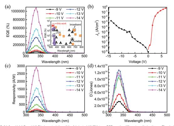
Fig. 2 (a) EQE, (b)  $J_d - V$ , (c) R, and (d)  $D^*$  characteristics of the fabricated UV PM-type OPDs under different applied voltages. The device structure is ITO/TAPC:  $C_{60}(50:1,80 \text{ nm})/Al(100 \text{ nm})$ . Inset of (a): summary of the peak EQEs of our prepared devices and the reported organic or organic/inorganic photodetectors.
