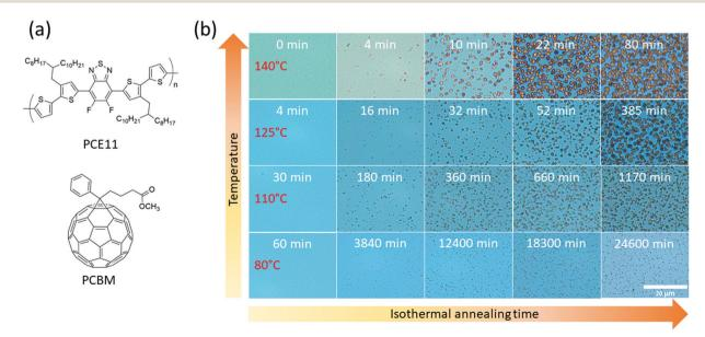
Fig. 1 (a) Chemical structure of PCE11 and PCBM. (b) Optical micrographs of PCE11:PCBM films between isothermal annealing steps at 140, 125, 110 and 80 °C, indicated at left column. Total annealing time is indicated on the top of each micrograph. The scale bar (20 µm) is equal for all micrographs.
