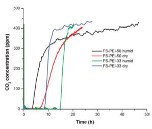
Fig. 9 Adsorption of CO<sub>2</sub> from the air at 25 °C on FS-PEI-50 and FS-PEI-33 under dry and humid conditions, illustrating longer period before breakthrough for FS-PEI-33 (33 wt% polyamine loading). Reprinted with permission from ref. 32 Copyright (2011) American Chemical Society.
