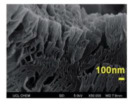
Fig. 5 SEM micrograph of exfGO-D\_7.0TETA, exfoliated graphene-oxide impregnated with 7.0 g g<sup>-1</sup> TETA. Reproduced from ref. 94 with permission from the Royal Society of Chemistry
