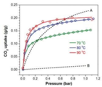
Fig. 15 CO<sub>2</sub> uptake isotherms of PEI-C60 at 70 °C, 80 °C and 90 °C and compared to the absorption of CO<sub>2</sub> on (A) Mg-MOF-74 and (B) MOF-177, both at 90 °C. Reproduced from ref. 106 according to Creative Commons Attribution 4.0 International (CC BY 4.0)
