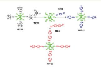
Fig. 7 Cross-linking of PEI with 2,4,6-tris(chloromethyl)mesitylene (TCM), 4,4'-bis-(chloromethyl)-1,1'-biphenyl (BCB), and p-dichloroxylene (DCX). Reprinted with permission from ref. 115. Copyright (2018) American Chemical Society
