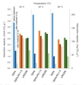
**Fig. 20** Effect of propylene oxide modification of TEPA- and PEHA-based adsorbents on  $CO_2$  adsorption under 95%  $CO_2$  in 25, 55, and 85 °C for 3 h before and after treatment under air or  $N_2$  at 100 °C for 20 h. Comparison with LPEI25k/50S. Reproduced with permission from ref. 70. Copyright 2019, John Wiley and Sons.
