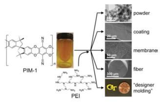
Fig. 6 PIM 1 as a solution-processable support for PEI and electron microscopy images show meso-/macroporosity engineered into final structure. Reprinted with permission from ref. 34. Copyright (2015) American Chemical Society
