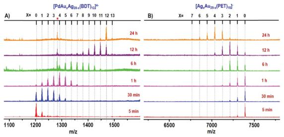
Fig. 4 Time-dependent ESI MS of intercluster reaction between PdAg<sub>28</sub> and Au<sub>25</sub> (1:5 ratio) where panel (A) shows the reaction at the PdAg<sub>28</sub> side and panel (B) presents the reaction at the  $Au_{25}$  side. The red asterisk corresponds to thiolates produced during the reaction. The species observed are  $[PdAu_xAg_{28-x}(BDT)_{12}]^{4-}$  and  $[Ag_xAu_{25-x}(PET)_{18}]^-$ . (reprinted with permission Copyright © 2019 American Chemistry Society). (10)
