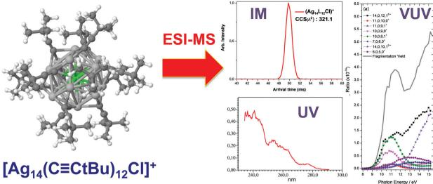
Fig. 11 DFT-optimized structures (chlorine, light green; silver, light gray; copper, orange; carbon, dark green; hydrogen, white) for  $[Ag_{14}(C \equiv CtBu)_{12}Cl]^{+}$ with lon-mobility arrival times (red peak) and optical action spectra in the UV and VUV range, (reprinted with permission Copyright® 2017 American Chemistry Society). 203
