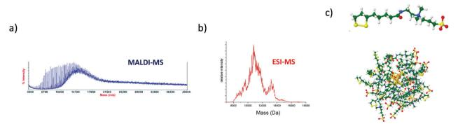
Fig. 5 (a) MALDI-MS and (b) Deconvoluted ESI-MS spectra of gold nanoclusters protected by multi-shells of thioctic bidentate zwitterionic ligands. (c) Possible structure for nanoclusters Au<sub>12</sub>Zw<sub>22</sub> (with thioctic-zwitterion ligand (Zw, C<sub>15</sub>H<sub>30</sub>N<sub>2</sub>O<sub>4</sub>S<sub>3</sub>). Adapted with permission Copyright() © 2017 AIP Publishing and  $\odot$  2014 and 2019 RSC Publishing).  $^{157,160,257}$
