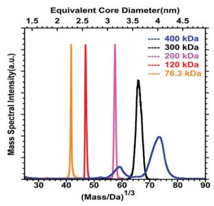
Fig. 2 MALDI-MS of 76.3 to 400 kDa nanoparticles synthesized using  $HSC_6H_{13}$  thiol. Mass spectrum data are plotted *versus* the cube root of mass to allow comparison with the core equivalent diameter (reprinted with permission Copyright© 2018 American Chemistry Society). 45
