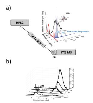
Fig. 7 (a) general online HPLC/ESI-MS setup. HPLC spectrum of the nanoparticles and corresponding mass spectra for each peak of elution (evidencing products of fragmentation and intact small rigid platform SRP NPs. (b) Chromatograms (HPLC-MS) recorded at different aging times of the solution. (reprinted with permission Copyright() 2013 American Chemistry Society). 159
