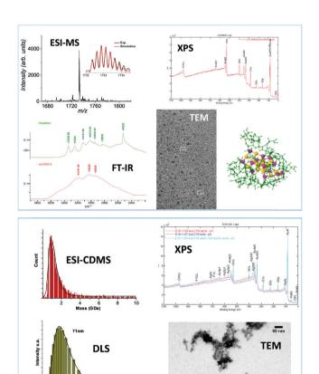
Fig. 12 Examples of characterization techniques in addition to mass spectrometry used for atomically precise  $Au_{15}SG_{13}$  nanoclusters (top panel) and Sub-100 nanometer silver doped gold-cysteine supramolecular assemblies (bottom panel). XPS: X-ray photoelectron spectroscopy, FT-IR: Fouriertransform IR spectroscopy, TEM: Transmission electron miscorscopy, DLS: dynamic light scattering.
