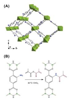
Fig. 1 (A) Representation of MIL-53(AI)-NH<sub>2</sub> structure in the open pore configuration, where AlO<sub>6</sub> polyhedra are depicted in green, and grey and navy are carbon and nitrogen atoms, respectively. (B) Scheme of postsynthetic modification of MIL-53(Al)-NH<sub>2</sub> structure with methyl methacrylic anhydride
