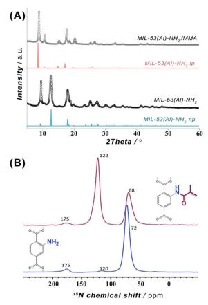
Fig. 2 (A) Powder XRD patterns of MIL-53(AI)-NH<sub>2</sub> nanoparticles before (black) and after (grey) post-synthetic modification with MMA and compared to open (lp) and narrow pore (np) forms. (B) Solid-state DNP-enhanced 15N NMR spectrum for MIL-53(Al)-NH<sub>2</sub> before (blue) and after (wine) postsynthetic modification with MMA.
