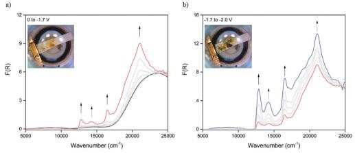
Fig. 2 Solid-state UV-Vis-NIR spectroelectrochemistry of 1 in 0.1 M  $[(n-C_aH_9)_4N]PF_6/DMF$  electrolyte showing potential changes from (a) 0 to -1.2 V and (b) -1.2 to -2.0 V where the arrows indicate the direction of the spectral progression. The step at 12500 cm<sup>-1</sup> is due to a detector change. Insets: Photographs of the sample acquired in situ during the time-course of the experiment.
