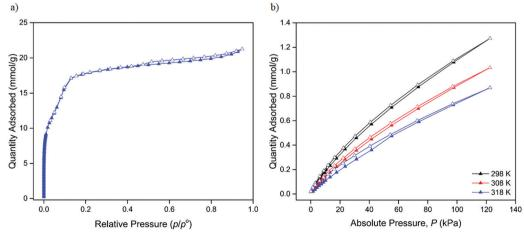
Fig. 3 Gas sorption isotherms of 1 showing adsorption of (a) N<sub>2</sub> at 77 K and (b) CO<sub>2</sub> at 298, 308 and 318 K. Adsorption and desorption are indicated by closed and open triangles respectively.
