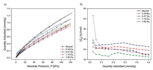
Fig. 5 (a) CO<sub>2</sub> adsorption (closed triangles) and desorption (open triangles) isotherms of the neutral and samples reduced by 0.39, 0.47, 1.15 and 1.82 equiv. of LiNP at 298 K and (b) CO2 isosteric heat of adsorption profiles for the neutral and chemically reduced samples.
