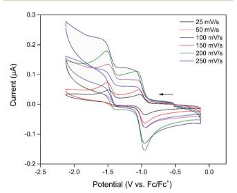
**Fig. 1** CV of **1** in 0.1 M  $[(n-C_4H_9)_4N]PF_6/DMF$  supporting electrolyte at scan rates of 25–250 mV s<sup>-1</sup>. The arrow indicates the direction of the forward scan.
