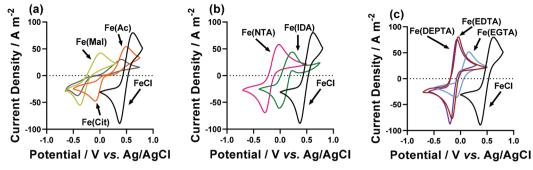
Fig. 4 Cyclic voltammograms of (a) Fe(Ac), Fe(Mal) and Fe(Cit), (b) Fe(IDA) and Fe(NTA) and (c) Fe(EDTA), Fe(EGTA) and Fe(DEPTA) redox couples; all are compared to the parent FeCl<sub>2/3</sub> species (i.e. 50 mM FeCl<sub>2</sub> and 50 mM FeCl<sub>3</sub>, in the absence of any ligand). All voltammograms were recorded at an Au working electrode, at a scan rate of 50 mV s<sup>-1</sup> and ambient temperature.
