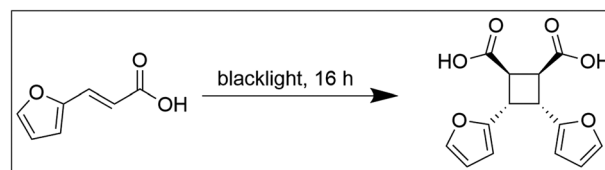
Fig. 1 Scheme of CBDA-2 synthesis from furfural derived trans -3-(2-furyl)acrylic acid.
