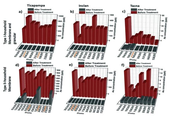
Fig. 4 Arsenic concentration before and after filtration through the type I household filtration unit in a) Ticapampa (H6), b) Inclan (H14), and c) Tacna (H3) and arsenic concentration before and after filtration through the type II household filtration unit in d) Ticapampa (H9), e) Inclan (H11) and f) Tacna (H1). The brown arrows indicate the date of the installation replacement.
