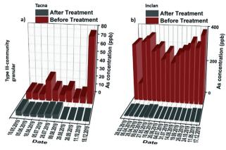
Fig. 5 Arsenic concentration before and after filtration through the type III community filtration unit in a) EPS Tacna and b) Inclan. According to the performance measured, there was no need to change the granular materials during the study.
