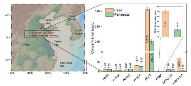
Fig. 5 Treatment of water sample from Xiaoging River basin by AM membrane. The map is generated from Schlitzer, Reiner, Ocean Data View, odv.awi.de, 2020. The removal efficiencies are summarized in the ESI† (Table S4).
