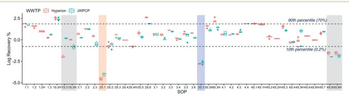
Fig. 2 Log-transformed OC43 recovery efficiency at Plant 1 (Hyperion) and Plant 2 (JWPCP), measured by each SOP. The SARS-CoV-2 results from the SOPs highlighted are not represented in Fig. 1 due to the fact that the results were all non-detect (gray), the recovery was below the quality control cut-off of 0.01% (blue), or both (orange).
