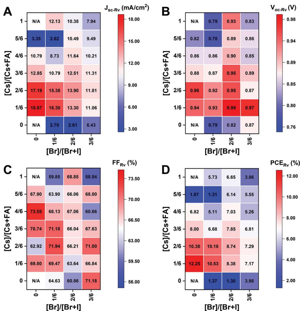
Fig. 10 Photovoltaic parameters of  $J_{sc}$  (A),  $V_{oc}$  (B), FF (C), and PCE (D) for the reverse scan obtained from the best devices of I-rich compositions using 0.4 M perovskite precursor solutions.
