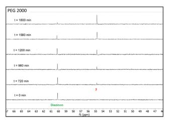
Fig. 6 Stacked <sup>31</sup>P-NMR spectra for the nucleophilic degradation of diazinon with piperidine performed in a mixture of 35 wt% PPG 400 + 15 wt% PEG 2000 + 50 wt% H<sub>2</sub>O at 298 K.
