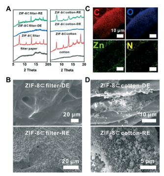
Fig. 3 (A) PXRD patterns of the degradation-reconstruction processes of ZIF-8 Cfilter and ZIF-8 Ccotton; SEM images of (B) ZIF-8 Cfilter after degradation and reconstruction and (D) ZIF-8 cotton after degradation and reconstruction; (C) EDS elemental mapping images of ZIF-8 Cfilter after degradation.
