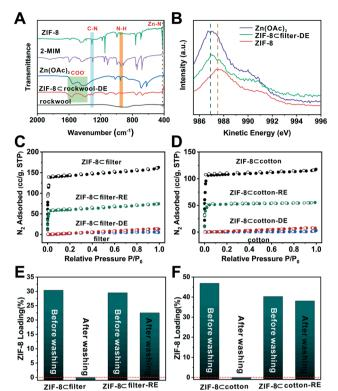
Fig. 4 (A) The FTIR spectrum of ZIF-8, 2-MIM, Zn(OAc)2, ZIF-8 Crockwool-DE and rockwool. (B) The Zn LMM Auger spectrum of Zn(OAc)<sub>2</sub>, ZIF⊂filter-DE and ZIF-8; 77 K N<sub>2</sub> sorption isotherms of (C) ZIF-8 cfilter and (D) ZIF-8 cotton during the degradationreconstruction cycle; ZIF-8 loading of (E) ZIF-8 ⊂ filter and ZIF-8 ⊂ filter-RE before and after washing and (F) ZIF-8 cotton and ZIF-8 cotton-RE before and after washing.
