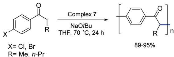
Scheme 8 Polymerization of 4-haloaryl alkyl ketones catalyzed by **7** as described by Matsubara and co-workers.<sup>27</sup>
