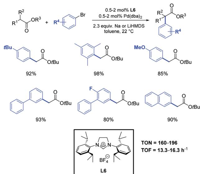
Scheme 31  $\alpha$ -Arylation of esters catalyzed by Pd(dba)<sub>2</sub> and **L6**, as described by Hartwig and co-workers.<sup>57</sup>
