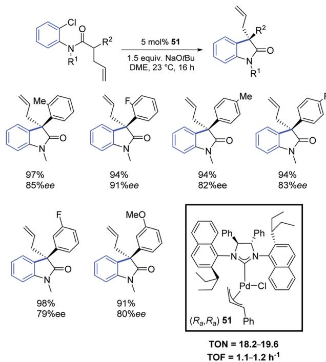
Scheme 38 Asymmetric oxindoles synthesis with (*R<sub>a</sub>,R<sub>a</sub>*)-**51** as described by Dorta.
