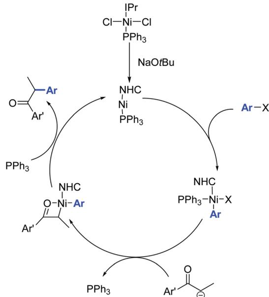
Scheme 20 Proposed mechanism for the  $\alpha$ -arylation of ketones in the presence of the Ni complex **34**, described by Matsubara and co-workers.<sup>46</sup>
