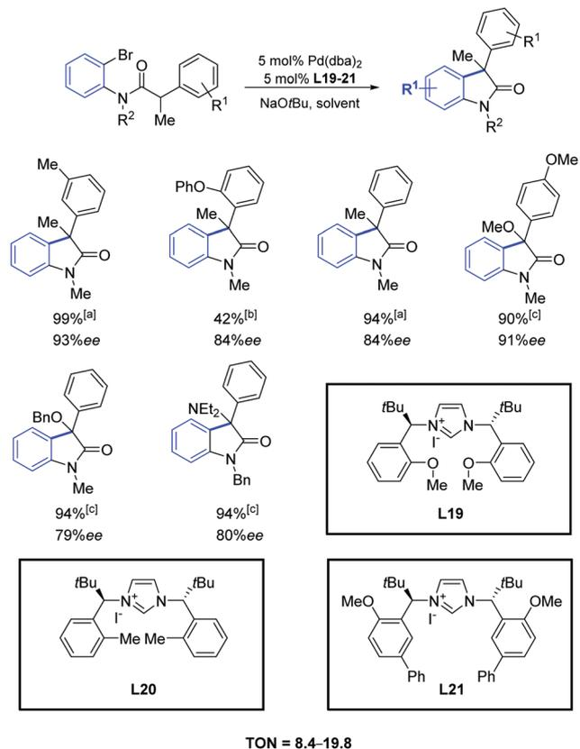
Scheme 36 Chiral azolium salts in the palladium catalyzed intramolecular cyclization of amides to oxindoles, as described by Küding and coworkers. <sup>a</sup>Ligand **L19**, DME, 23 °C; <sup>b</sup>Ligand **L20**, DME, 23 °C; <sup>c</sup>Ligand **L21**, toluene, 50 °C.
