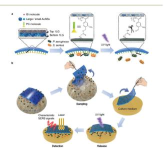
**Fig. 5** Schematic illustration of (a) SERS adhesive tape for pathogen capture and release and (b) pathogen sampling from skin wound, photo-controlled release to solid culture medium for pathogen growth, and *in situ* SERS detection of *S. aureus* and *P. aeruginosa*. The image is reprinted from Guo *et al.*, <sup>99</sup> Copyright (2019), with permission from American Chemical Society.
