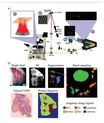
Fig. 3 Multi-foci Raman spectroscopy to reduce multimodal spectral histopathology (MSH) measurement speeds: (a) the LC-SLM (1) generates multiple laser foci on the sample surface (2) and the DMD (3) generated conjugated reflective pinholes, with collected light being dispersed onto a CCD inside the spectrometer (4); (b) example of a multi-foci MSH measurement performed on a frozen BCC-positive skin specimen (Reproduced from ref. 71 with permission from © The Optical Society, copyright 2016).
