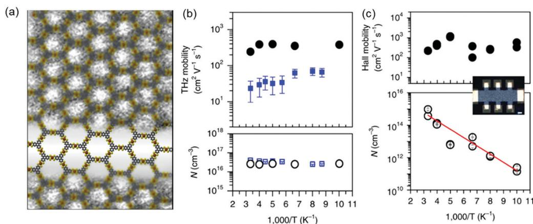
Fig. 18 (a) A high-resolution transmission electron microscopy image of the  $\text{Fe}_3(\text{THT})_2$  2D conjugated MOF together with the structural schematic (grey, yellow and orange: carbon, sulfur and iron atoms, respectively). (b and c) Charge transport studies by THz spectroscopy and Hall effect measurements, respectively. Scale bar: 100  $\mu\text{m}$ . Reproduced with permission from ref. 132. Copyright 2018 Nature Publishing Group.
