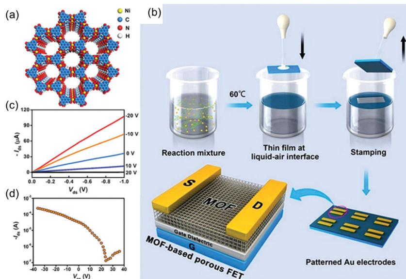
Fig. 15 (a) Schematic structure of semiconducting Ni<sub>3</sub>(HITP)<sub>2</sub>. (b) Schematic illustration of the fabrication of Ni<sub>3</sub>(HITP)<sub>2</sub> film-based porous FETs. (c and d) Output curves and transfer curve for the Ni<sub>3</sub>(HITP)<sub>2</sub>-based FET, respectively. Reproduced with permission from ref. 164. Copyright 2017 American Chemical Society.
