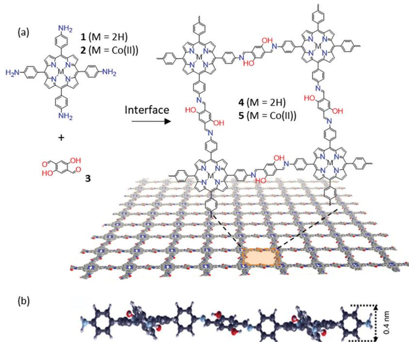
Fig. 2 (a) Chemical structures of monomers (**1**, **2**, and **3**) and 2D polymers (**4** and **5**). (b) The cross-sectional view of the molecular structure of a monolayer 2DP (**4**) suggested by DFTB. Reproduced with permission from ref. 34. Copyright 2016 Nature Publishing Group.
