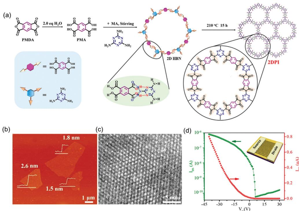
Fig. 11 (a) Solvothermal synthesis of 2D polyimide nanosheets. (b) AFM image. (c) HRTEM image. (d) Transfer curve of the 2D polyimide-based FET device ( $V_{DS} = 1$  V). Reproduced with permission from ref. 87. Copyright 2019 American Chemical Society.
