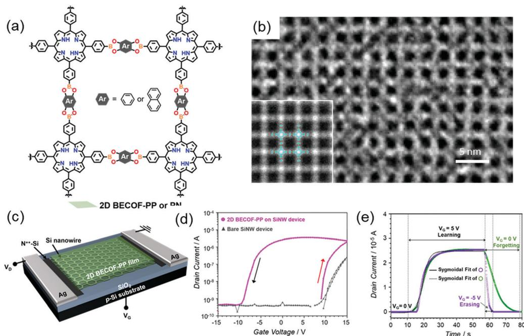
**Fig. 17** (a) Chemical structure of the boronate ester-based 2D COFs. (b) HR-TEM image. The inset is a lattice-averaged image calculated from DFT. (c) Schematics of the 2D COF/SINW hybrid device. (d) Transfer characteristics of the hybrid device. (e) Learn-erase/learn-forget cycles. Reproduced with permission from ref. 37. Copyright 2020 Wiley & Sons.
