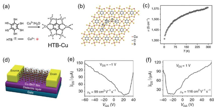
**Fig. 14** (a) Schematic synthesis of the HTB-Cu MOF. (b) Schematic structure of the 2D lattice of HTB-Cu with cell parameters of  $a = b = 8.76 \text{ \AA}$ . (c) Variable-temperature conductivity measurement on a  $150 \text{ nm}$  film by the in-line four-probe method. (d) Illustrative scheme of the HTB-Cu-based FET. (e and f) Output characteristics of the HTB-Cu-based FET. Reproduced with permission from ref. 142. Copyright 2015 Nature Publishing Group.
