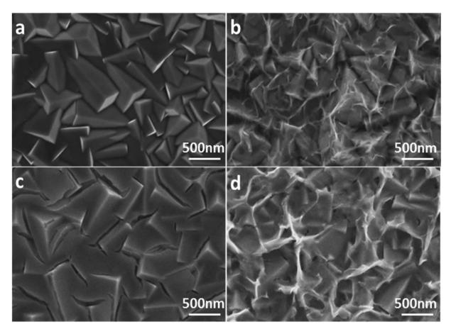
Fig. 1 Top-view SEM images of (a) bare Cu<sub>2</sub>O, (b) ZnO/Cu<sub>2</sub>O, (c) TiO<sub>2</sub>/Cu<sub>2</sub>O, and (d) TiO<sub>2</sub>/ZnO/Cu<sub>2</sub>O photoelectrodes.
