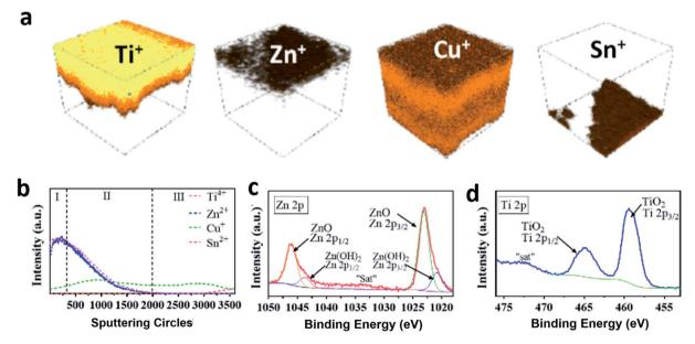
Fig. 3 (a) 3D elemental rendering images and (b) corresponding XPS depth profile of the  $TiO_2/ZnO/Cu_2O$  composite structure by TOF-SIMS. Core-level XPS spectra of (c) Zn 2p for the  $ZnO/Cu_2O$  photoelectrode and (d) Ti 2p for the  $TiO_2/ZnO/Cu_2O$  photoelectrode. The remark of "sat" means the satellite peak.
