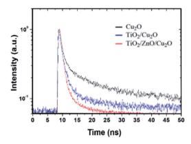
Fig. 5 Time-resolved PL spectra acquired with an excitation wavelength of 405 nm for the prepared Cu<sub>2</sub>O (black), TiO<sub>2</sub>/Cu<sub>2</sub>O (blue) and TiO<sub>2</sub>/ZnO/Cu<sub>2</sub>O (red) photoelectrodes.
