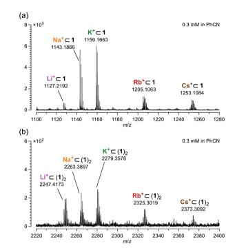
Fig. 4 Mass spectra of (a)  $M^+ \subset 1$  and (b)  $M^+ \subset (1)_2$  measured using a benzonitrile solution on ESI method.
