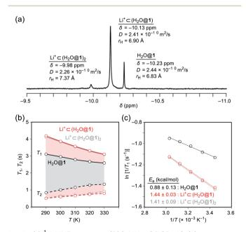
Fig. 7 (a)  $^1$ H NMR spectrum (500 MHz, ODCB- $d_4$ ), (b) temperature dependence of relaxation times (errors less than 5%), and (c) Arrhenius plots (ln  $1/T_1$  vs. 1/T) of H<sub>2</sub>O@1 with 20 equiv. of Li<sup>+</sup>[B(C<sub>6</sub>F<sub>5</sub>)<sub>3</sub>] $^- \cdot 2.5$ Et<sub>2</sub>O (800 MHz, ODCB- $d_4$ ).
