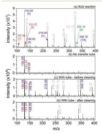
Fig. 10 Mass spectra for the Hantzsch synthesis conducted in the bulk (a) and in ESSI droplets with no transfer tube (b), with a 55 cm tube before cleaning (c) and after cleaning with acetone wash (d). Label color (same as in eqn (8)): red = reagents, purple = reaction intermediates, green = product, grey = peaks from impurities. In parentheses the labels for each reagent, intermediate and product molecule from eqn (8); all ions are  $[M+H]^+$ .
