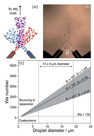
Fig. 6 Schematics (a) and still frame (b) from Lee  $et~al.^{46}$  showing the microdroplet fusion mass spectrometry setup. (c) Weber number (We) calculated for the collision of two equally-sized aerosol droplets with variable colliding angle,  $\theta$ ; the diameter range of  $13 \pm 6~\mu m$  indicated by Lee  $et~al.^{46}$  is shown for reference. The horizontal dashed line at We = 150 separates regions where coalescence or bouncing/separation are expected to occur.
