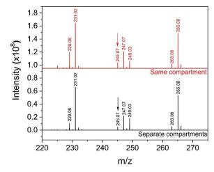
Fig. 8 Mass spectra from the reaction of ribosylation of uracil with the reagents in the same compartment' setup (a) and the reagents in separate compartments' configuration (b). The peak at m/z=245.07 was previously assigned to uridine<sup>21</sup> and is indicated with an arrow; the full peak attribution can be found in Table S1.†
