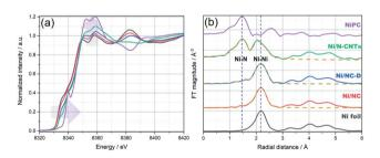
Fig. 3 (a) Normalized XANES spectra and (b) Fourier transform (FT) of  $k^2$ -weighted EXAFS (solid lines) and the fit results (dashed lines) for Ni foil (black), Ni/NC (red), Ni/NC-D (blue), Ni/N-CNTs (green), and Ni-PC (purple), respectively. The blue vertical dashed lines at ca. 1.45 and 2.19 Å in (b) are to mark the position of Ni-N and Ni-Ni bonds, respectively. Details on the EXAFS analysis are provided in the ESI.†
