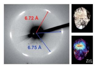
Fig. 3 (Left) Hexagonal six-fold X-ray diffraction pattern obtained for the functionalized nanothread; and (right)  $50 \times$  images within a stainless-steel gasket, illustrating crystallinity along with (bottom) a polarized light micrograph using a 530 nm waveplate.
