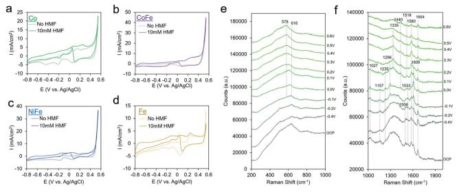
Fig. 5 Extension to other transition metal thin films. Co (a), CoFe (b), NiFe (c), and Fe (d) catalysts were screened for their activity towards HMF oxidation. A closer look at AuCo catalysts with operando Raman spectroscopy in the low frequency region reveals the formation of an amorphous CoO<sub>x</sub> surface under oxidizing conditions<sup>35</sup> (e), and the high-frequency region gives insight on the nature of the surface intermediates (f).
