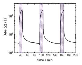
Fig. 5 Absolute value of impedance Z of the  $H_2O@Cu_2(SP-BPDC)_2(dabco)$  sample at 1 Hz versus time. The sample is irradiated with UV light for 10 min each.
