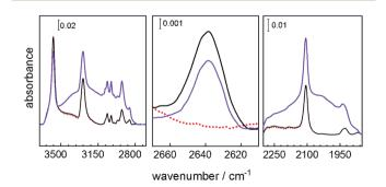
Fig. 6 Infrared spectra of the  $Cu_2(SP\text{-BPDC})_2(dabco)$  SURMOF. The spectrum of the empty SURMOF is shown as red dotted line, the  $D_2O$ -loaded SURMOF in the spiropyran form is shown as black solid line and in the merocyanine form as violet line. The center panel shows the band of  $D_2O$  valence vibration. The panel on the right- and left-hand side show the vibration of the H-bonded and D-bonded species. The entire infrared spectra are shown in Fig. SI6.†
