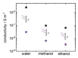
Fig. 4 Conductivity of water, ethanol and methanol in  $\text{Cu}_2(\text{SP-BPDC})_2(\text{dabco})$  SURMOF with the photoswitchable groups in the spiropyran form (black) and in the merocyanine form (violet). The experiments (Fig. 3 and SI5†) are repeated three times. The average values and the standard deviations as error bars are shown here.
