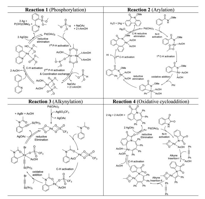
Scheme 2 Key steps involved in the catalytic cycles for reactions 1-4, shown using a monometallic Pd species.
