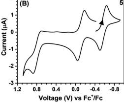
Fig. 2 Cyclic voltammograms of 1 (A) and 5 (B). Arrow denotes scan direction. Conditions: DCM, 0.1 M [TBA][PF $_6$ ], 0.1 V s $^{-1}$ .
