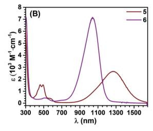
Fig. 4 UV-vis-NIR absorption spectra of 1–3 (A), 5 and 6 (B) in DCM. Concentration: 1, 92  $\mu$ M; 2, 3, 5 and 6, 50  $\mu$ M.
