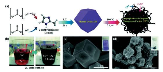
Fig. 7 Synthesis of a Co/Zn hybrid MOF and nano-porous carbon. (a) Preparation of Co/Zn (2:1) hybrid-ZIF from a metal precursor and 2-methylimidazole organic linker followed by carbonization to produce graphitic and amorphous nanoporous carbons. (b) Pictures of 2 L-scale production. SEM images of (c) a bimetallic Co/Zn hybrid ZIF and (d) carbonized nano-porous carbon. Reproduced with permission from the Royal Society of Chemistry ref. 78, copyright 2016.
