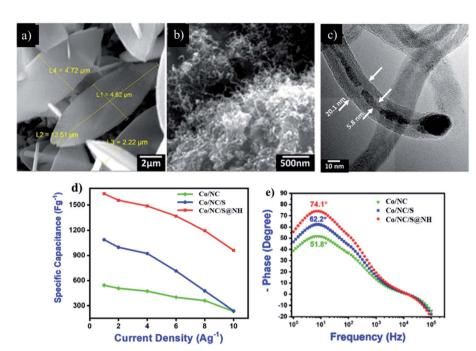
Fig. 9 SEM images of before (a) and after (b and c) the synthesis of ZIF-67 derived n-doped CNTs decorated with sulfur and nickel hydroxide, (d) specific capacitance calculated from CV curves as a function of scan rate for the Co/NC, Co/NC/S, and Co/NC/S@NH electrodes, (e) Bode phase angle plots of synthesized electrodes on Ni foam. Reproduced with permission from Elsevier, ref. 40, and Copyright 2020.
