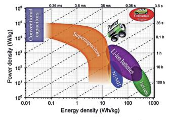
Fig. 1 Ragone plots of different energy storage systems.<sup>6</sup>
