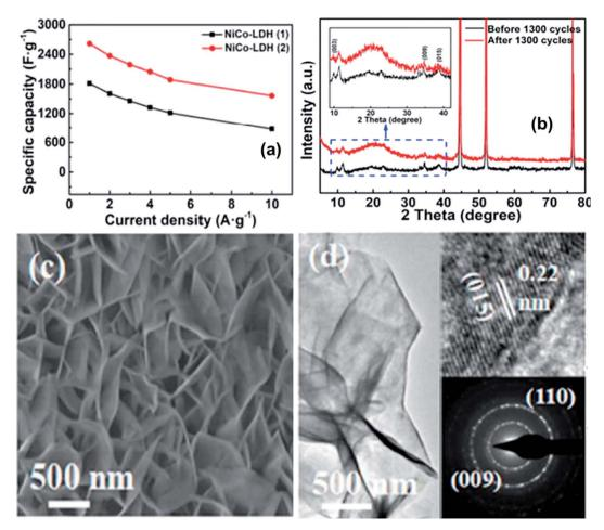
Fig. 11 (a) Specific capacitance of NiCo-LDH/NF ( $\alpha$  and  $\beta$ ) at different current densities; (b) retention capacity; (c) comparison of the XRD patterns of NiCo-LDH/NF ( $\beta$ ) before and after the life cycles; (c and d) SEM and TEM images of NiCo-LDH/NF, respectively. Reproduced with the approval from ref. 24, Copyright 2019, Elsevier.
