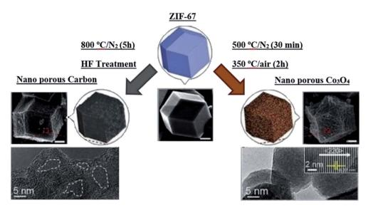
Fig. 8 Representation of the preparation of nanoporous carbons and nano-porous Co<sub>3</sub>O<sub>4</sub> from ZIF-67 as a precursor, which shows the retention of the morphology of the parent ZIF-67, as shown in the SEM and TEM images. Reproduced with permission from American Chemical Society, ref. 35, Copyright 2015.
