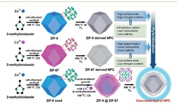
Fig. 4 Production of ZIF-8 and ZIF-67-derived nanoporous carbon and its advantages and disadvantages. Reproduced with permission from the American Chemical Society, ref. 63, Copyright 2015.
