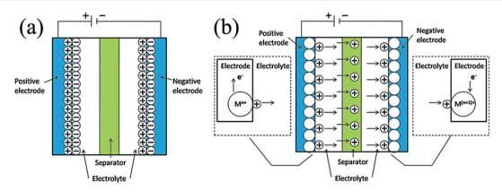
Fig. 2 Representation of various supercapacitors: (a) electrical double-layer capacitors (EDLCs); (b) pseudo-capacitors (PCs) (where M exemplifies a metal atom; if electrolyte anions participate in reversible redox reactions, they move in the opposite route to the cations).<sup>14</sup>
