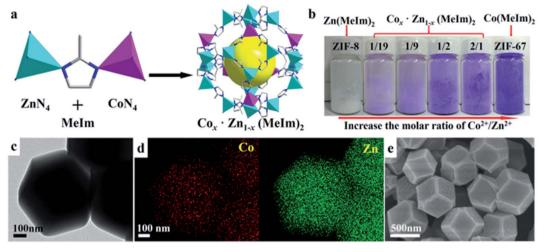
Fig. 6 (a) Preparation of Zn/Co-ZIFs and (b) colors of Zn/Co-ZIFs with various compositions; (c) TEM image, (d) elemental mapping and (e) SEM image of Zn/Co-ZIFs. Reproduced with permission from ref. 72, Copyright 2016, Nature Publishing Group.
