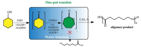
Fig. 2 Schematic representation of the synthesis of the oligomer (ε-caprolactone) via an enzyme cascade.<sup>26</sup>
