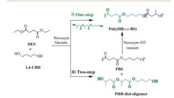
Fig. 5 Schematic of bio-based poly(3-hydroxybutyrate-co-butylene succinate) synthesized by enzymatic polycondensation via a one-step or two-step Process.83
