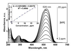
Fig. 4 UV absorption spectra of methyl red (MR) in 0.25 M H<sub>2</sub>SO<sub>4</sub> solution as a function of MR concentration in the range of 2–20 mg L<sup>-1</sup>. Inset: Beer law applied to the principal absorption bands located at 520 nm.
