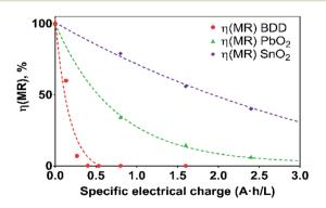
Fig. 7 Current efficiency ( $\eta$ ) values for the electrooxidation of MR as a function of the specific electrical charge (A h L<sup>-1</sup>) for solutions containing 20 mg L<sup>-1</sup> MR in 0.5 M H<sub>2</sub>SO<sub>4</sub> at 30 mA cm<sup>-2</sup> and 298 K: • Si/BDD, • Ti/Sb-doped SnO<sub>2</sub>, • Pb/PbO<sub>2</sub>.
