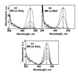
Fig. 5 UV-vis spectra for 20 mg  $L^{-1}$  MR solutions in 0.5 M  $H_2SO_4$  electrolyzed at 30 mA cm<sup>-2</sup> and 298 K, as a function of the electrolysis time and the material of anode: (a) Pb/PbO<sub>2</sub>, (b) Si/BDD and (c) Ti/Sb-doped SnO<sub>2</sub>.
