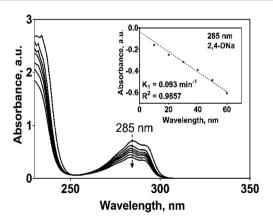
Fig. 12 UV spectra, as a function of the electrolysis time, for 100 mg  $\rm L^{-1}$  2,4-DNa solutions in 0.5 M NaClO $_4$  electrolyzed on a Si/BDD anode at 30 mA cm $^{-2}$  and 298 K. Inset shows the pseudo-first order graphic of the UV band decrease at 285 nm.
