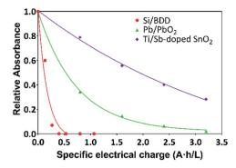
Fig. 6 Plots of the relative absorbance of MR again specific electrical charge (A h L<sup>-1</sup>) for solutions containing 20 mg L<sup>-1</sup> MR in 0.5 M H<sub>2</sub>SO<sub>4</sub> at 30 mA cm<sup>-2</sup> and 298 K:  $\bullet$  Si/BDD,  $\bullet$  Ti/Sb-doped SnO<sub>2</sub>,  $\blacktriangle$  Pb/PbO<sub>2</sub>.
