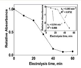
Fig. 9 Plot of the relative absorbance at 285 nm of 2,4-DNa as a function of the electrolysis time for the electrolysis of a solution containing 100 mg  $L^{-1}$  2,4-DNa in 0.5 M  $\rm Na_2SO_4$  at 30 mA cm $^{-2}$  and 298 K on Si/BDD anode. Inset shows the corresponding pseudo-first order graphic.
