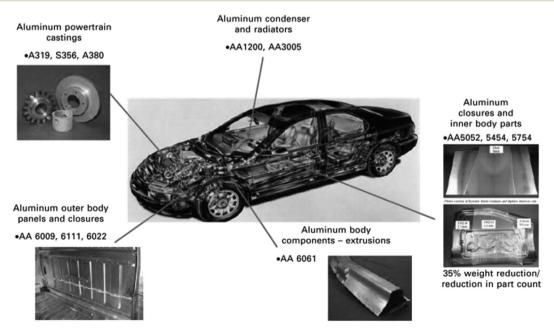
Fig. 12 Application of different series of aluminum alloys in automotive product forms. This figure has been reproduced from ref. 92 with permission from Elsevier, copyright 2010.
