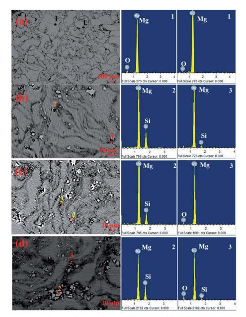
Fig. 10 (a-d) SEM micrographs with EDS spectra: (a) pure Mg, (b) Mg-1Si, (c) Mg-4Si and (d) Mg-6Si. This figure has been reproduced from ref. 17 with permission from Elsevier, copyright 2020.
