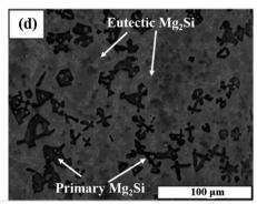
Fig. 7 SEM micrographs of Mg-5 wt% Si alloys (a) without modifier, (b) 5 wt% Kg-5 Kg-5 Kg-5 Kg-5 Wt% KBF $_4$  + Kg-5 Kg-5
