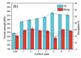
Fig. 9 The tensile strength (TS) and elongation (strain %) of the Al–Mg–Si alloy *versus* Conform pass: (a) after 1 to 7 Conform processes (N) and (b) after 1 to 7 Conform processes followed by aging at 175 °C for 8 h. This figure has been reproduced from ref. 73 with permission from Elsevier, copyright 2017.
