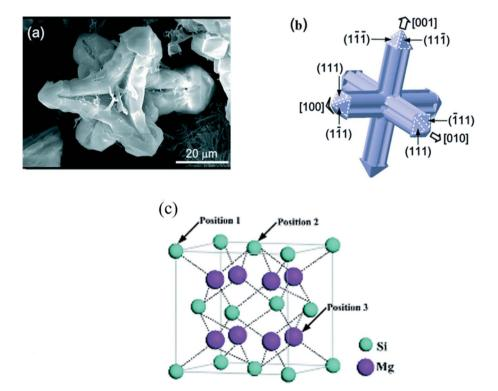
Fig. 3 (a and b) Structure and planes of the primary  $Mg_2Si$  phase. (c) Molecular structure of the  $Mg_2Si$  phase. This figure has been reproduced from ref. 23 with permission from Royal Society of Chemistry, copyright 2014.
