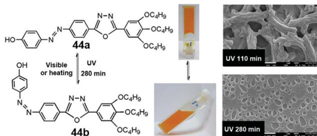
Fig. 18 Structures of **44a–b** and their dichloromethane gel ( $2.0 \text{ mg mL}^{-1}$ ) before (top) and after (bottom) UV irradiation and the SEM images (right). Reproduced with permission.<sup>54</sup> Copyright 2015, Royal Society of Chemistry.
