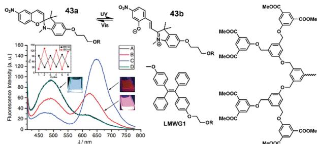
**Fig. 17** Structures and fluorescence spectra of the organogel formed with **LMWG1** (10 mM) and **43a** (10 mM) in toluene (A) after UV-light (365 nm) irradiation for 30 s (B) and 10 min (C) and subsequent visible-light (550 nm) irradiation for 10 min (D);  $\lambda_{\text{exc}} = 400$  nm. Reproduced with permission.<sup>53</sup> Copyright 2010, Wiley-VCH.
