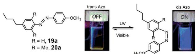
Fig. 8 Structures of **19a** and **20a**, and visualized images of photoswitchable fluorescence "on/off" behavior of **19a**. Reproduced with permission.<sup>34</sup> Copyright 2012, Royal Society of Chemistry.
