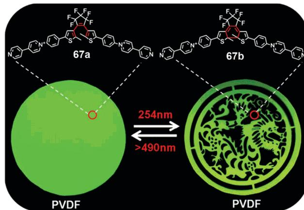
Fig. 33 Fluorescent photographs of **67a**-embedded PVDF film under alternating 254 nm UV- and visible-light irradiations. Reproduced with permission.<sup>81</sup> Copyright 2018, American Chemical Society.
