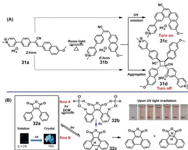
Fig. 12 (A) Chemical structures of **31a–d** and their corresponding photochromic mechanisms. (B) Chemical structures of **32a–c** and their AIE and photochromic properties. Reproduced with permission.<sup>43</sup> Copyright 2017, Royal Society of Chemistry.
