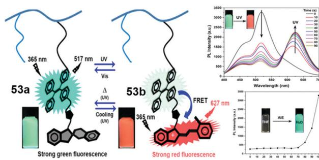
Fig. 24 Schematic illustration of the energy transfer from the TPE to MC unit *via* the FRET process after UV exposure and the AIE property of **53a** in  $THF/H_2O$  solutions. Reproduced with permission.<sup>65</sup> Copyright 2020, American Chemical Society.
