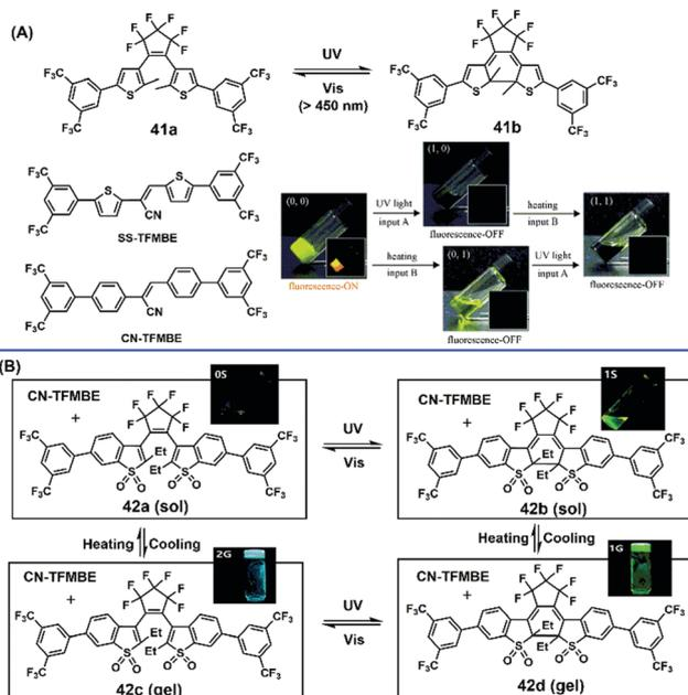
**Fig. 16** (A) Photochromic reaction of **41a** and illustration of binary logic gate. Reproduced with permission.<sup>51</sup> Copyright 2009, Wiley-VCH. (B) Schematic illustration of **42a** and photographs of their four states. Reproduced with permission.<sup>52</sup> Copyright 2018, Wiley-VCH.
