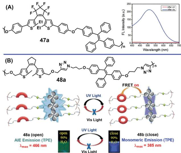
Fig. 21 (A) Structure of polymer **47a** and reversible fluorescence switching of the polymer film using UV and visible light. Reproduced with permission.<sup>60</sup> Copyright 2016, Royal Society of Chemistry. (B) Structure of polymer **48a** and pictorial diagram of **48a** from its opened to closed form upon UV irradiation. Reproduced with permission.<sup>61</sup> Copyright 2017, Royal Society of Chemistry.
