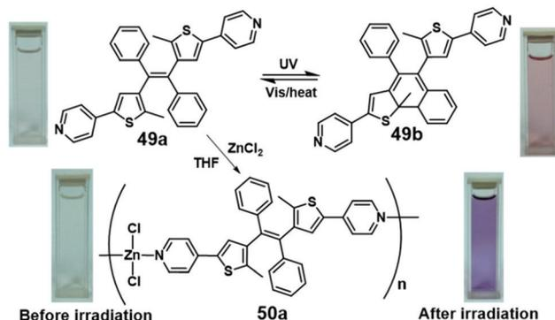
Fig. 22 Photochromic reactions and correlative color changes of monomer **49a** and polymer **50a**. Reproduced with permission.<sup>62</sup> Copyright 2018, Chemical Society of Japan.
