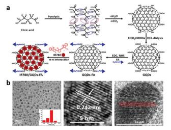
Fig. 2 (a) Schematic illustrating the preparation of IR780/GQD-FA. Reprinted with permission from ref. 20. Copyright 2017 American Chemical Society. (b) TEM image and HRTEM image with the measured lattice spacing and the sp<sup>2</sup> domain of the GQDs. Reprinted with permission from ref. 20. Copyright 2017 American Chemical Society.
