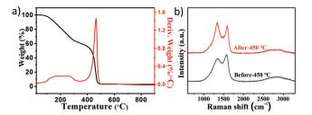
Fig. 2 (a) TG and DTG curves of the mixed product in the range of 20-900 °C under airflow. (b) Raman spectra of the mixed product before and after heated at 450 °C.
