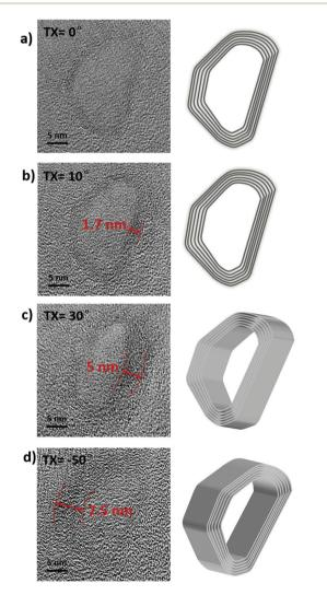
Fig. 4 TEM images and projection images of the polyhedral H-CNOs observed with tilting angles of (a) 0, (b) 10, (c) 30, and (d) -50 degrees.
