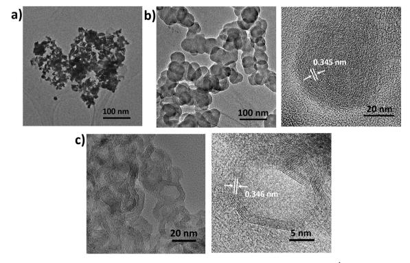
Fig. 3 TEM images of the collected products by ultrasonic dispersion in CHP for 1 h at a concentration of 1  $\mu$ g mL<sup>-1</sup>, and centrifugation at (a) 6000 rpm, (b) 8000 rpm and (c) 12 000 rpm.
