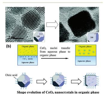
Fig. 4 (a) Transmission electron microscopy (TEM) images of the evolution from CeO<sub>2</sub> truncated nanooctahedra to nanocube. (b) Schematic illustration of shape evolution of CeO2 nanocrystals in the organic phase. Adapted with permission from ref. 47 Copyright 2010, American Chemical Society..
