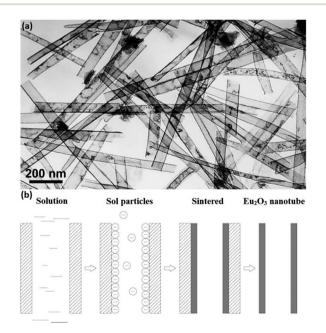
Fig. 7 (a) TEM image of Eu<sub>2</sub>O<sub>3</sub> nanotubes. (b) Schematic illustration of the formation mechanism of Eu<sub>2</sub>O<sub>3</sub> nanotubes. Adapted with permission from ref. 54. Copyright 2004, American Chemical Society.
