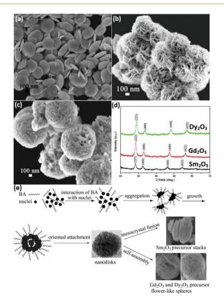
Fig. 10 SEM images of (a) Sm<sub>2</sub>O<sub>3</sub> nanodisks; (b) Gd<sub>2</sub>O<sub>3</sub>; and (c) Dy<sub>2</sub>O<sub>3</sub> flower-like spheres. (d) XRD patterns and (e) schematic illustration of the possible formation process of Sm<sub>2</sub>O<sub>3</sub> nanodisks or Gd<sub>2</sub>O<sub>3</sub> and Dy<sub>2</sub>O<sub>3</sub> flower-like spheres. Adapted with permission from ref. 66. Copyright 2009, American Chemical Society.
