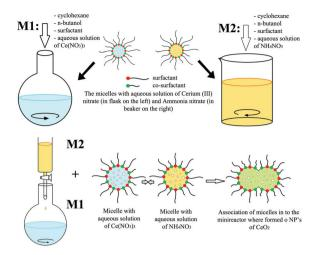
Fig. 5 Schematic illustration of the synthesis of CeO<sub>2</sub> nanoparticles via precipitation in reverse microemulsions. Adapted with permission from ref. 53. Copyright 2019, Springer Nature.
