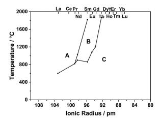
Fig. 2 Phase diagram of RE<sub>2</sub>O<sub>3</sub>.
