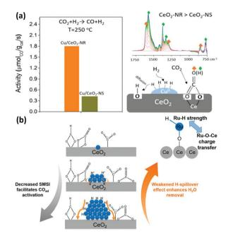
Fig. 16 (a) Activity and schematic illustration of the mechanism of the RWGS reaction for Cu/CeO<sub>2</sub> nanorods and Cu/CeO<sub>2</sub> nanospheres. Adapted with permission from ref. 94. Copyright 2018, American Chemical Society. (b) Schematic illustration of the compete effect between SMSI and H-spillover on Ru/CeO2 catalysts for the CO2 methanation reaction. Adapted with permission from ref. 96. Copyright 2018, American Chemical Society.
