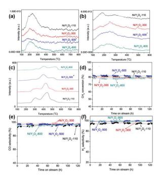
Fig. 19 (a) NH<sub>3</sub>-TPD profiles of the Ni/Y<sub>2</sub>O<sub>3</sub> samples. (b) CO<sub>2</sub>-TPD profiles of the Ni/Y<sub>2</sub>O<sub>3</sub> samples. (c) TPR profiles of the Ni/Y<sub>2</sub>O<sub>3</sub> samples. Catalytic performance of the Ni/Y<sub>2</sub>O<sub>3</sub> samples in the partial oxidation of methane: (d) CH<sub>4</sub> conversion; (e) CO selectivity; and (f) H<sub>2</sub> selectivity. Adapted with permission from ref. 117. Copyright 2014, Elsevier.
