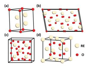
Fig. 1 Schematic illustration of the crystal structure of rare earth oxides: (a) A-type RE<sub>2</sub>O<sub>3</sub>, (b) B-type RE<sub>2</sub>O<sub>3</sub>, (c) C-type RE<sub>2</sub>O<sub>3</sub>, and (d) fluorite REO<sub>2</sub>.
