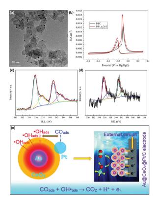
Fig. 20 (a) TEM image of Pd-La<sub>2</sub>O<sub>3</sub>/C. (b) Cyclic voltammograms of Pd/C and Pd-La<sub>2</sub>O<sub>3</sub>/C in 1 M KOH + 1 M CH<sub>3</sub>OH. XPS spectra of Pd 3d for (c) Pd/C and (d) Pd-La<sub>2</sub>O<sub>3</sub>/C. Adapted with permission from ref. 129 Copyright 2019, Elsevier. (e) Schematic illustration of the possible mechanism of Au@CeO2@Pt/C for the MOR. Adapted with permission from ref. 130. Copyright 2019, Royal Society of Chemistry.
