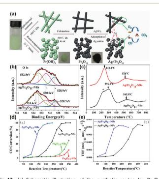
Fig. 13 (a) Schematic illustration of the synthetic routes for  $Pr_6O_{11}$ nanostructures. (b) O 1s XPS spectra of  $Ag/Pr_6O_{11}$  catalysts. (c)  $H_2$ -TPR profiles of  $Ag/Pr_6O_{11}$  catalysts. (d) CO conversion of  $Pr_6O_{11}$  and Ag/Pr<sub>6</sub>O<sub>11</sub> samples for CO oxidation. (e) TOF of Pr<sub>6</sub>O<sub>11</sub> and Ag/Pr<sub>6</sub>O<sub>11</sub> samples for CO oxidation. Adapted with permission from ref. 79. Copyright 2017, American Chemical Society.
