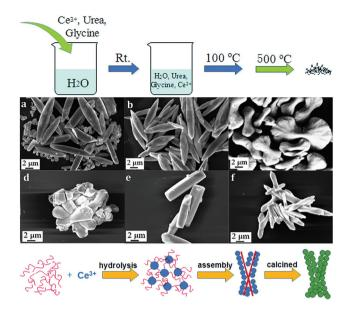
Fig. 11 (a) Procedure for the synthesis of 3D porous CeO<sub>2</sub>. SEM images of CeO<sub>2</sub> prepared with different ratios of reagents (Ce<sup>3+</sup>: urea: glycine) of (b) 3:0:1; (c) 3:1:1; (d) 3:2:1; (e) 3:40:1; (f) 3:4:2; and (g) 6:2:1. (h) Schematic illustration of the formation of the 3D porous CeO<sub>2</sub> with a bowknot shape. Adapted with permission from ref. 44. Copyright 2018, Royal Society of Chemistry.
