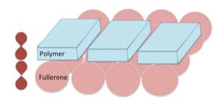
Fig. 12 Representation of the different orientations of polymer donor and fullerene acceptor units in a thin solid film, in which the aromatic core of the polymer units is considered as a relatively flat building block for simplicity. Schematic orientation of the  $\pi$ -orbitals is indicated (brown p orbitals). In the left structure triplet formation by charge recombination will be enhanced due to orthogonal  $\pi$ -orbitals.
