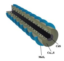
Fig. 4 Schematic illustration of the crystal structure of heterointerfaces. Copyright 2020, American Chemical Society. Reprinted from ref. 34 with permission.
