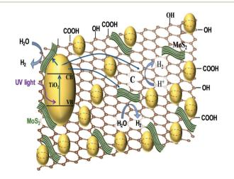
Fig. 1 Schematic illustration of photocatalytic activity of the TiO<sub>2</sub>/ MoS<sub>2</sub>/graphene nanocomposite.
