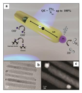
Fig. 3 (a) Illustration of the NP photocatalyst depicting the photocatalytic cycle. (b) TEM and (c) high-resolution HAADF micrographs of a few representative Pt tipped CdSe@CdS rods. Copyright 2016, American Chemical Society. Reprinted from ref. 32 with permission.
