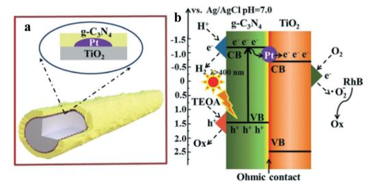
Fig. 6 Schematic structure (a) and the photogenerated electron-hole transfer pathways (b) inside the CN/Pt/TiO2 composite under visible light irradiation. Copyright 2019, Royal Society of Chemistry. Reprinted from ref. 39 with permission.
