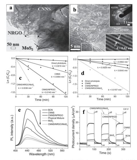
Fig. 7 (a and b) TEM images, SAED pattern, and HRTEM images of CNNS/NRGO/MoS<sub>2</sub> nanojunctions, (c and d)  $ln(C_t/C_0)$  of MB and Cr(vi) versus time for different photoactive materials under simulated sunlight irradiation, (e) PL spectra and (f) transient photocurrent density versus Na<sub>2</sub>SO<sub>4</sub> electrolyte. Copyright 2013, Wiley Online Library. Reprinted from ref. 53 with permission.
