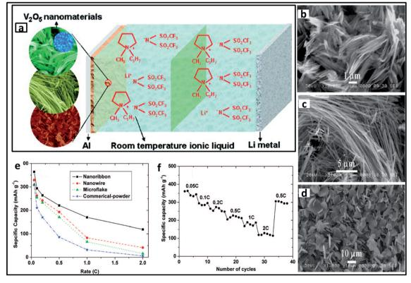
Fig. 15 (a) Schematic representation of a lithium metal battery using  $V_2O_5$  nanomaterials and room temperature ionic liquid electrolyte. SEM images of diverse morphologies of  $V_2O_5$  materials: (b) nanoribbons (c) nanowires (d) microflakes and their corresponding (e) specific capacities; (f) cycle life of V<sub>2</sub>O<sub>5</sub> nanoribbon. "Adapted with permission from ref. 218. Copyright (2008) American Chemical Society."
