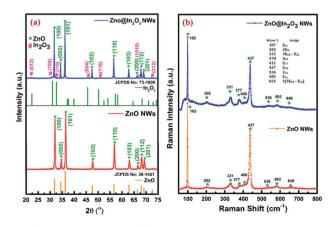
Fig. 1 (a) XRD patterns and (b) Raman spectra of ZnO nanowires and ZnO@ $\ln_2O_3$  heterojunction nanowires.
