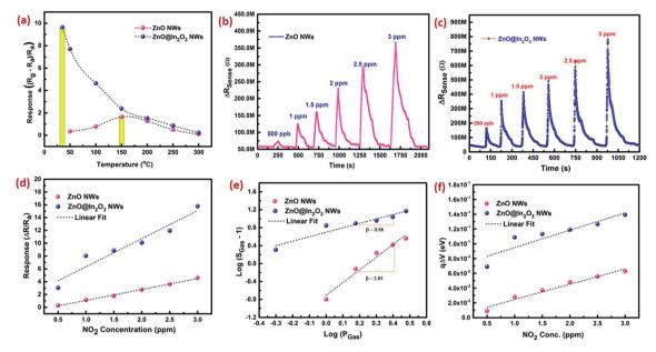
Fig. 5 (a) Response towards exposure to 1 ppm of NO<sub>2</sub> as a function of temperature, (b and c) dynamic NO<sub>2</sub> sensing characteristics, (d) NO<sub>2</sub> response graph, (e)  $\log(S_{Gas} - 1)$  against  $\log P_g$  plot of curves and (f) variations in the band bending energy graph of ZnO nanowires and ZnO@In<sub>2</sub>O<sub>3</sub> heterojunction nanowire based sensors.
