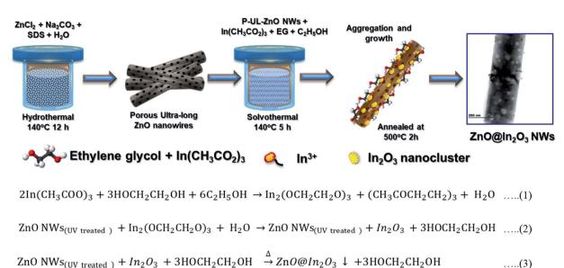
Scheme 1 Schematic diagram of the synthesis method adopted for n-n type  $ZnO@ln_2O_3$  heterojunction nanowires.
