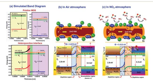
Scheme 3 (a) Simulated energy band diagram before and after contact and schematic diagram showing the  $NO_2$  sensing mechanism (b) in air atmosphere and (c) in the  $NO_2$  gas atmosphere, deduced for  $ZnO@ln_2O_3$  heterojunction nanowires.
