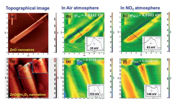
Fig. 6 Representative AFM topographical images of (a) ZnO nanowires and (d) ZnO@ $ln_2O_3$  heterojunction nanowires (inset shows the magnified image of heterojunction nanowires), (b and c) SKPM images of ZnO nanowires in air and the NO $_2$  environment and (e and f) SKPM images of ZnO@ $ln_2O_3$  heterojunction nanowires in air and NO $_2$  environments (inset shows the CPD in air and the NO $_2$  environment).
