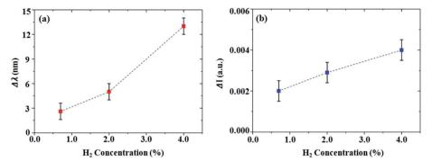
Fig. 5 Variation of experimental (a) wavelength shift,  $\Delta\lambda$ , and (b) reflectance intensity change of reflection minima,  $\Delta I$ , observed in the AZO nanotube sensing system in the presence of H<sub>2</sub> gas of different concentrations (0.7%, 2%, and 4%). Here the dotted lines are for guidance to see how  $\Delta\lambda$  and  $\Delta I$  change for different concentrations of H<sub>2</sub> gas.
