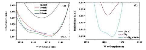
Fig. 6 (a) Response of the AZO nanotube sensing system over time in the presence of 4% H<sub>2</sub> gas. It is very clear that 10 min is enough to detect the presence of 4% H<sub>2</sub> gas. (b) The response of the AZO nanotube sensing system (with the PMMA channel) in the presence and absence of N<sub>2</sub> gas where there is almost no variation in the mode. But a clear shift of the mode is observed in the presence of 4% H<sub>2</sub> gas after 60 min.
