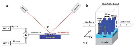
Fig. 2 (a) Schematic diagram of the experimental set-up. (b) Schematic diagram of the AZO nanotube sensing system.
