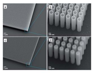
Fig. 1 Scanning electron microscope (SEM) images of the fabricated AZO (a, b) nanotubes and (c, d) pillar structures with a pitch of 400 nm, diameter of 300 nm, and height of 2  $\mu$ m. The wall thickness of nanotubes is approximately 20 nm.
