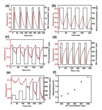
Fig. 5 Dynamic response-recovery curves of the gas sensor based on uranium dioxide nanoparticles towards (a) 20 ppm NO<sub>2</sub>; (b) 1000 ppm EtOH; (c) 1000 ppm CO; (d) 500 ppm NH<sub>3</sub>; and (e) varying CO concentration; (f) CO sensing response as a function of gas concentration. For measuring the NO<sub>2</sub> response, a 200 sccm N<sub>2</sub> flush was used for 1 h to recover the baseline.
