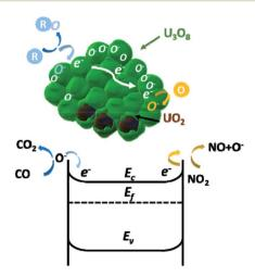
Fig. 8 Gas sensing mechanism of  $UO_2/U_3O_8$  nanoparticles when exposed to oxidizing and reducing gases.
