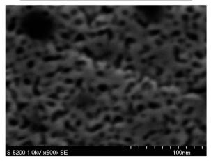
Fig. 2 (a) SEM image of electrochemically dealloyed NPG. (b) SEM image of white gold leaf dealloyed in nitric acid. (c) SEM image of electrochemically dealloyed NPG-Pt.
