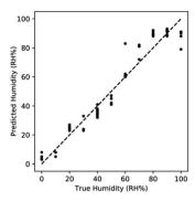
Fig. 10 Performance of kNN regression utilizing both features for AuAgPt. Sensing improves when combining features, with non-linearity manifesting at high RH% due to saturation.
