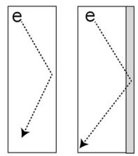
Fig. 1 Electron scattering at the ligament surface is the primary resistance to conduction in NPG and is strongly modulated by the substances adsorbed on the surface.
