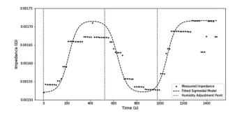
Fig. 8 Estimations of instantaneous impedance by STFT analysis during humidity changes. Dotted lines indicate humidity cycling between 5% and 95%. Sensor response is stable and returns to the original values. The transition time between equilibrium states was  $\sim 200 \text{ s}$ .
