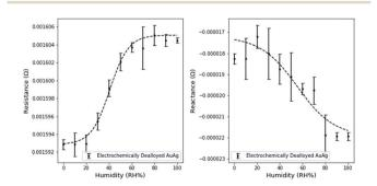
Change in electrical characteristics with variations in humidity levels. Resistance and reactance are associated with the in and out of phase signal response respectively. Data was fitted to a scaled sigmoidal curve
