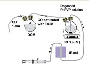
**Scheme 1** Acquisition of FTIR spectra of CO adsorbed on the Pt NP surface.
