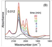
Fig. 7 Sets of time-course FTIR spectra of CO adsorbed on 1.4 nm-diameter Pt:PVP particles acquired after (A) 6.0 h or (B) 0.5 h of dissolution in DCM.
