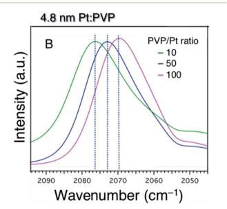
Fig. 6 FTIR spectra of 4.8 nm-diameter Pt:PVP particles subjected to 20 min of purging with CO and consisting of various molar ratios of PVP monomer to Pt atoms as indicated.
