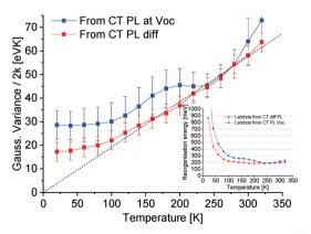
**Fig. 5** Normalized variance of Gaussian fits from the TAPC(6%): $C_{60}$  CT-state dominated emission obtained from the PL at OC or the spectra obtained from evaluating the difference between  $PL_{OC}-PL_{SC}$  as shown in Fig. 4. Inset shows the corresponding apparent reorganization energies obtained by dividing the normalized Gaussian variance by the temperature. For the subtracted spectra, a fairly constant reorganization energy is found for  $T>120\,$  K.
