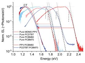
Fig. 2 Normalized electroluminescence spectra of some classical pure OPV materials and blends on logarithmic scale, emphasizing the varying slope of the high-energy tail. Dashed lines are fits to the well-known relation in eqn (5), whereas the dotted lines are accounting only for the exponential part of the same equation.
