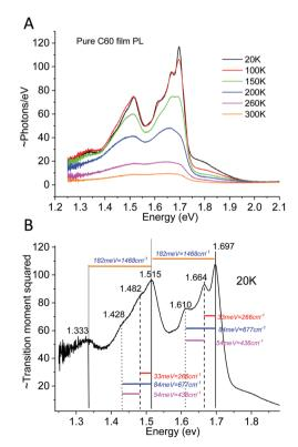
Fig. 3 (A) Temperature dependent PL emission (photon flux per eV) from pure films of  $C_{60}$ . (B) 20 K spectra divided by  $E^3$  rendering the relevant distribution proportional to the transition moment squared. The stiff intramolecular bond stretching completely governs the vibrational progression<sup>35</sup> of the spectra, whose dominant vibrational energies are designated.
