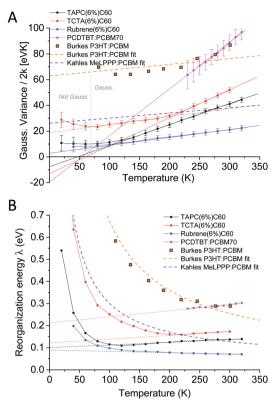
(A) Temperature dependence of the obtained Gaussian variance of the  $E^3$  reduced spectra from the electroluminescence in Fig. 6. (B) The corresponding ("apparent") reorganization energy, determined by dividing the data in (A) with the temperature. Whereas Burke's EQE and Kahle's PL data showed strongly T-dependent reorganization energies (almost constant variance dominated by static disorder) our data do not indicate any pronounced contribution to line-width broadening from static disorder.
