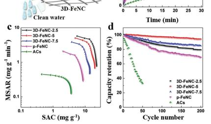
Fig. 6 (a) Schematic representation of the possible CDI process in oxygenated saline water using 3D-FeNC tubes. (b) SAC variations, (c) CDI Ragone plots, and (d) CDI cycling performances of 3D-FeNC-y (y = 2.5, 5 and 7.5), p-FeNC, and ACs in oxygenated saline water (5 mM).
