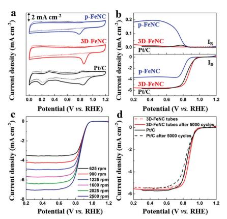
Fig. 5 (a) CV and (b) LSV curves of p-FeNC, 3D-FeNC, and Pt/C catalysts at 1600 rpm in  $N_2$  (dot line)/ $O_2$  (solid line)-saturated 0.1 M KOH solution. (c) LSV curves of the 3D-FeNC catalyst in  $O_2$ -saturated 0.1 M KOH solution at different rotating speeds. (d) LSV curves of the 3D-FeNC and Pt/C catalysts before and after 5000 cycles in  $O_2$ -saturated 0.1 M KOH solution at 1600 rpm. The scan rate is 10 mV s<sup>-1</sup> for LSV curves in (b-d).
