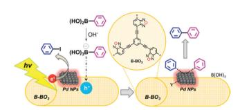
**Fig. 15** Organic/inorganic hybrid structure of CPPs for electron transfer. Heterojunction formation between poly(benzoxadiazole) and palladium nanoparticles. Reproduced with permission. Copyright 2015 American Chemical Society.
