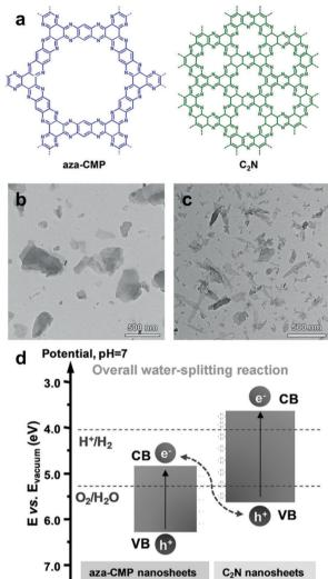
Fig. 14 Organic hybrid structure of CPPs for energy band alignment. (a) Chemical structure of aza-conjugated microporous polymer (aza-CMP) and  $C_2N$  nanosheets. TEM images of the exfoliated (b) aza-CMP and (c)  $C_2N$  nanosheet. (d) Electronic band structures of aza-CMP and  $C_2N$  nanosheet for a Z-scheme heterostructure. Reproduced with permission. Copyright 2018 Wiley-VCH.
