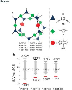
Fig. 10 HOMO/LUMO controls in CPPs by varying the amount of electron withdrawing units. (a) Synthetic compositions of D–A based conjugated nanoporous polymers, P-BBTs and (b) their redox potentials measured by cyclic voltammetry vs. SCE (Saturated Calomel Electrode). Reproduced with permission.<sup>98</sup> Copyright 2016 Wiley-VCH.
