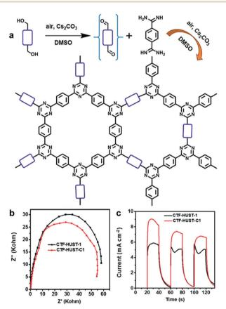
Fig. 9 Crystallinity of CPPs for charge transport. (a) Synthetic scheme of crystalline CTF-HUST-1 through in situ formation of aldehyde monomer from alcohol monomer. (b) Electrochemical impedance spectroscopy Nyquist plots and (c) photocurrent responses of the crystalline CTF-HUST-C1 and the layered CTF-HUST-1. Reproduced with permission.<sup>95</sup> Copyright 2018 Wiley-VCH.
