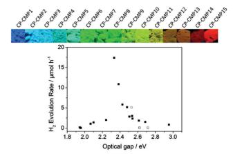
Fig. 4 Statistical copolymerization of comonomers for band gap engineering of CPP. Pyrene-based conjugated microporous polymers and their photocatalytic H<sub>2</sub> production efficiencies. Reproduced with permission.<sup>28</sup> Copyright 2015 American Chemical Society.
