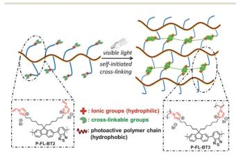
Fig. 20 Functionality control of CPPs for water compatibility. Conjugated polymer networks with vinylimidazolium group for self-initiated crosslinking. Adapted with permission. <sup>128</sup> Copyright 2015 Wiley-VCH.
