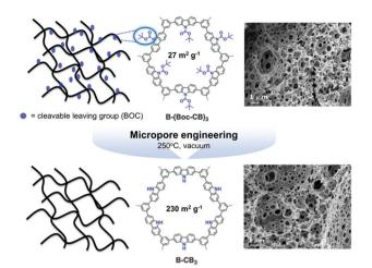
Fig. 19 Porosity control of CPPs by thermal deprotection of the functional group. Generation of additional porosity via a thermal deprotection of the BOC group in  $\pi$ -conjugated polyHIPEs. Reproduced with permission.<sup>23</sup> Copyright 2014 The Royal Society of Chemistry.
