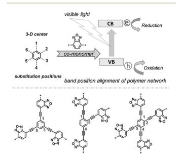
Fig. 7 Substitution geometry effect for charge transport in CPPs. Structural design of poly(benzoxadiazole)s by changing the substitution position on the central phenyl ring with benzoxadiazole linkers. Adapted with permission.<sup>26</sup> Copyright 2015 Wiley-VCH.
