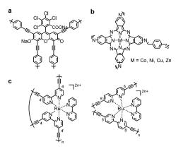
Fig. 3 Incorporation of photosensitizers in CPPs for light harvesting. (a) Conjugated microporous polymer with Rose Bengal Dye (RB-CMP1) and (b) metallophthalocyanine (MPc-CMP, M = Co, Ni, Cu, Zn). (c)  $Ru(bpy)_3^{2+}$ homocoupled polymers containing high Ru(bpy)<sub>3</sub><sup>2+</sup> loading up to 90%.
