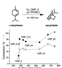
Fig. 17 Porosity control of CPPs by the silica template. Photocatalytic conversion of  $\alpha$ -terpinene into ascaridole with poly(benzothiadiazole)s having difference surface areas. Photo-reactor set-up with (a) lower  $O_2$  flow rate (5 mL min<sup>-1</sup>) and (b) higher  $O_2$  flow rate (10 mL min<sup>-1</sup>). Adapted with permission.<sup>22</sup> Copyright 2013 Wiley-VCH.
